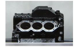
Marine Outboard, Snowmobile, Motorcycle and other similar cylinders can be easily mounted and rolled over for precision blind hole honing.
