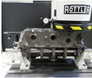
Extra clearance below and behind the fixture allow high deck height V-Blocks to be rolled to both banks for surfacing without removing the block from the machine.
