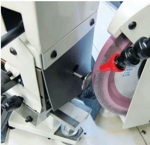
The VR12 allows very small diameter and short valves to be reground.
