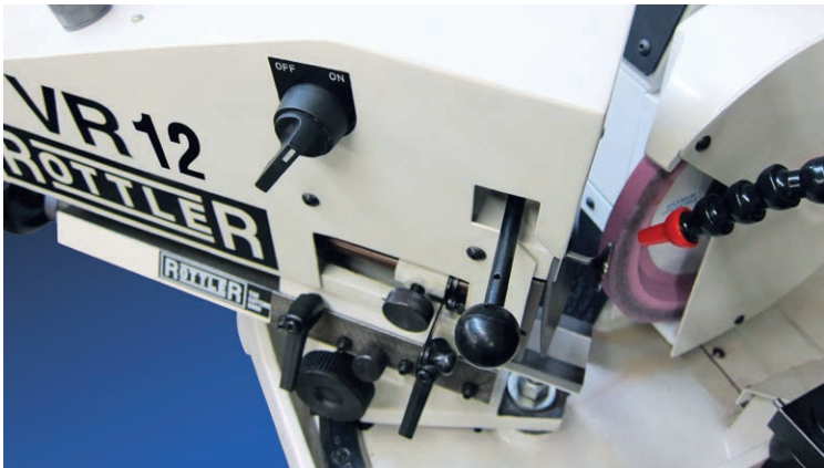
The VR12 allows very small diameter and short valves to be reground.
